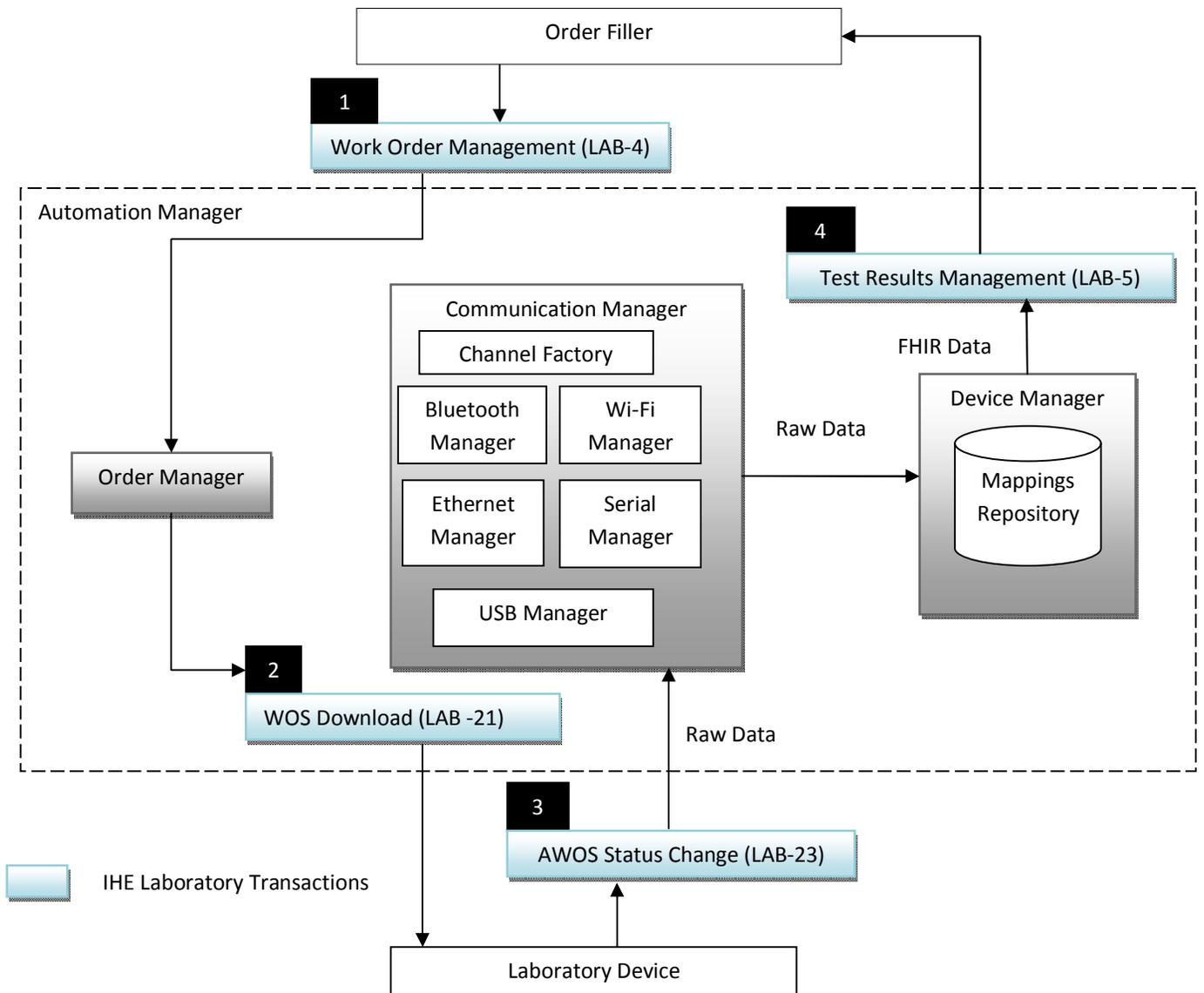
Fig. 5. Architecture of Medical Device Interoperability Middleware
