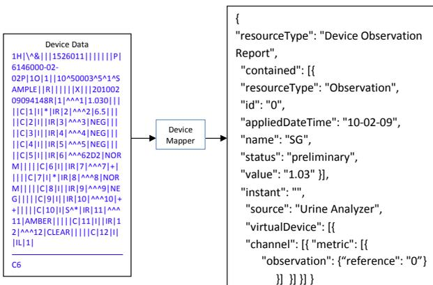
Fig. 6. Result of Urine Analyzer
