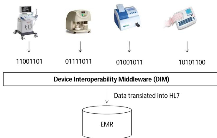
Fig. 1. High Level Architecture of the Middleware
